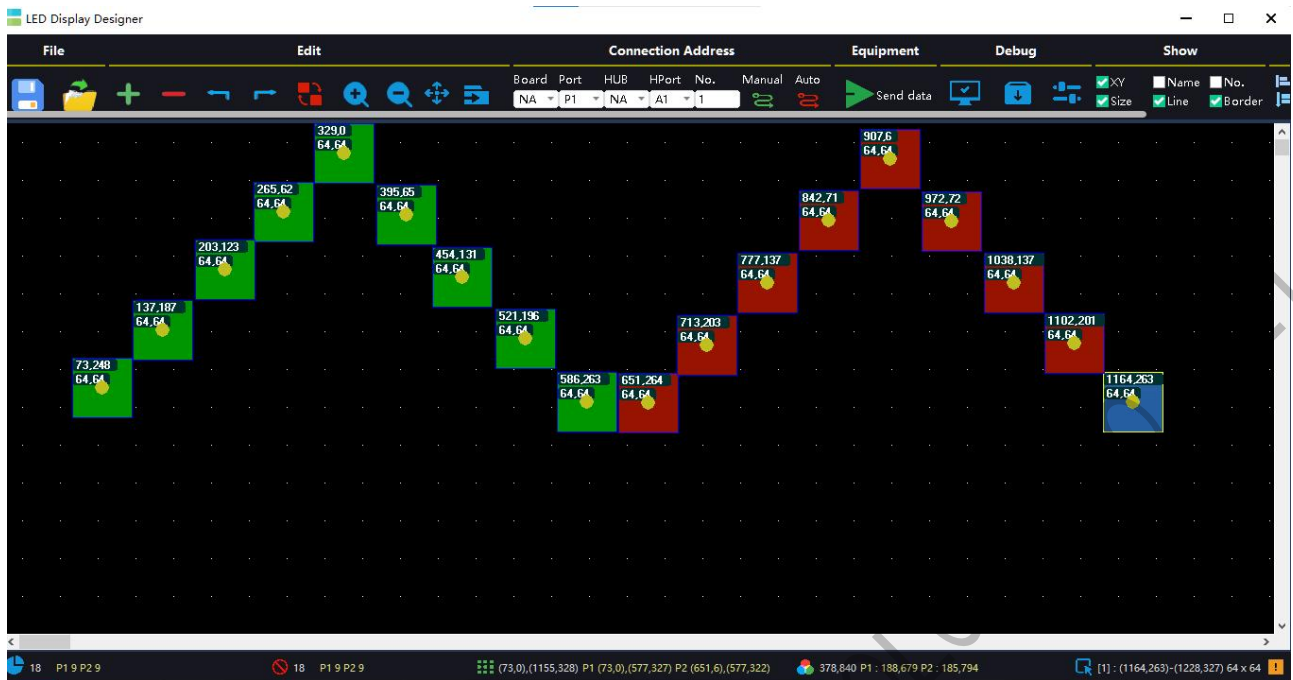
Figure 4-3-7 Set the connection sequence of receiving card
