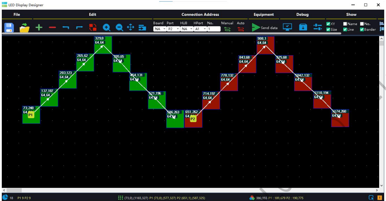
Figure 4-3-8 The serial number setting of the network port receiving card
